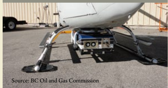
Exhibit 19: Helicopter with methane detector mounted on the underside
